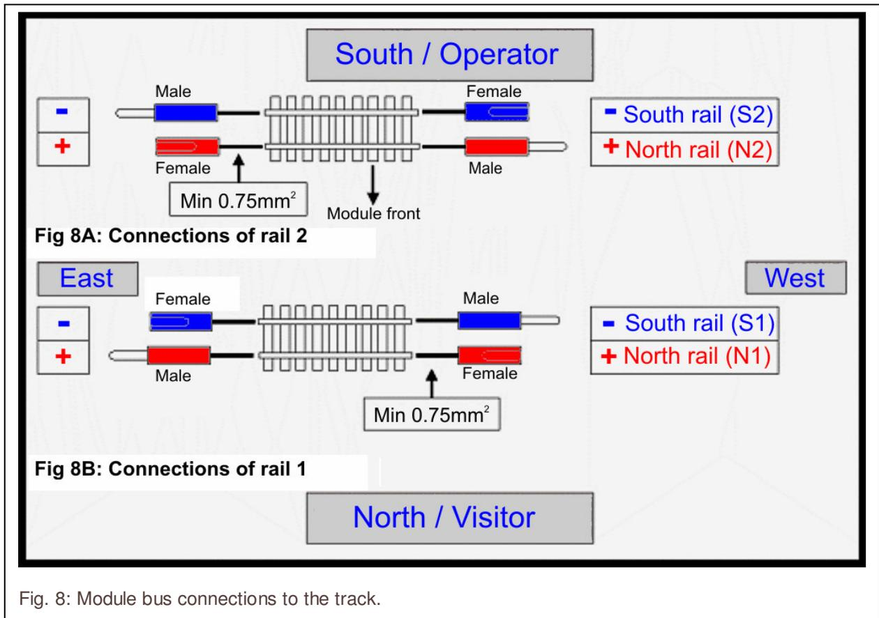
Fig. 8: Module bus connections to the track.
