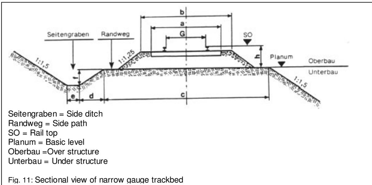
Nm gauge dimensions in millimeters:  $G = 6.5$ ,  $a = 12$ ,  $b = 14$ ,  $c = 26$ ,  $d = 5$ ,  $e = 2$ ,  $f = 1.5$  and  $h = 6$ .
