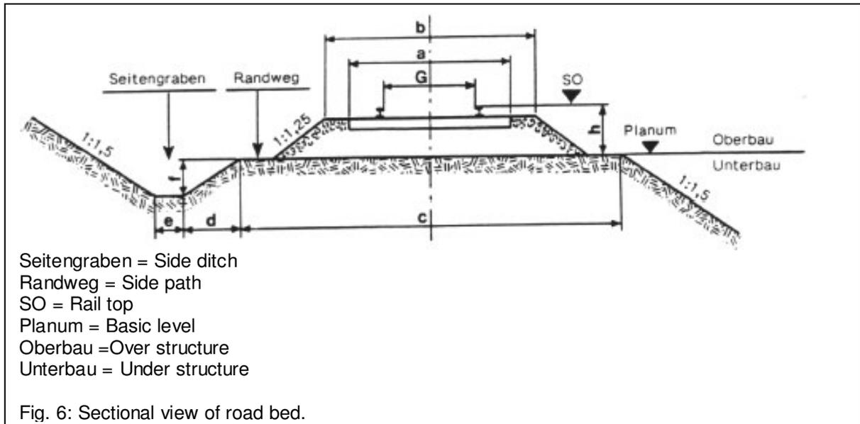
N scale dimensions in millimeters:  $G = 9$ ,  $a = 16$ ,  $b = 22$ ,  $c = 38$ ,  $d = 5$ ,  $e = 3$ ,  $f = 3$  and  $h = 6$ .
